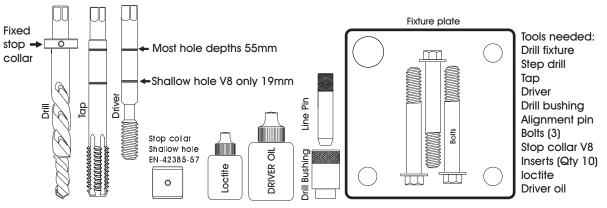
NOTE: A Special Stop collar EN-42385-57 is required on 1 upper left shallow hole on the V8 Block
