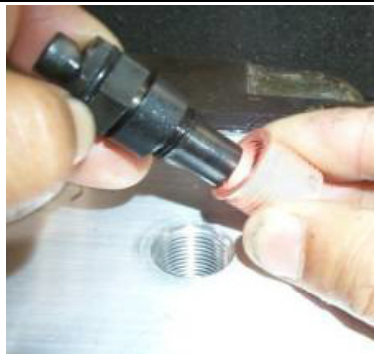
A: Screw the setting tool into the insert.
