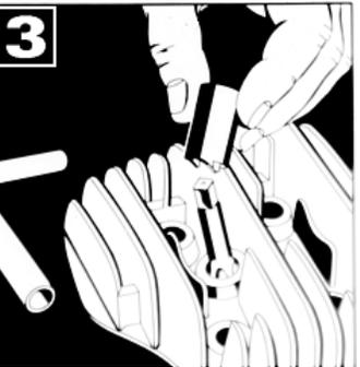
**3. Leave the step tap in the hole. Place the seat cutter over the shank.** The seat cutter does 2 operations. First the seat cutter will cut the counter sink for the flange of the insert, then it cuts a seat.
