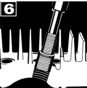
**6. Note: Tapered Seat inserts silver plated and require sealer p/n 6020 on external threads. Using the wrench provided rotate the driver through the insert. When the insert is seated the driver will tighten up. With increased pressure continue to rotate the driver through the insert until it loosens up. Then back the driver tool out of the insert.**
